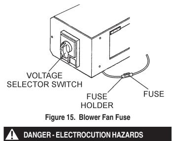
This fuse has current running through it any time the engine is running. This fuse is **NOT** connected to the main circuit breaker of the generator. Attempting to replace the fuse
